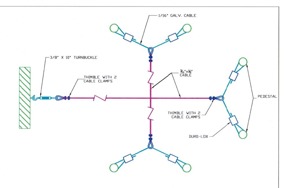
TEE JOINT DUCT - UNDER FLOOR MOUNTING
