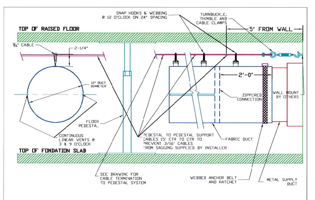
UNDERFLOOR FABRIC DUCT-SINGLE CABLE/SNAP HOOK MOUNTING
