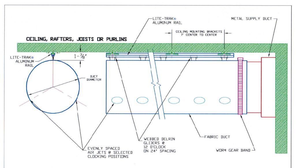
SINGLE CEILING MOUNT/SNAP HOOK AND FABRIC DUCT ATTACHMENT
